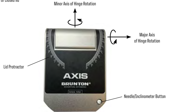
FIGURE 2: Diagram of closed lid
