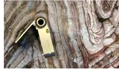
FIGURE 28: Using the Axis as a field protractor to measure angles between fold limbs (pictured) or conjugate fractures.
